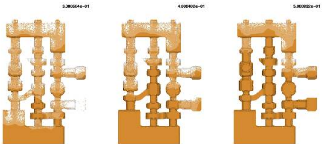
Figure 12. This illustrates core filling sequence.
