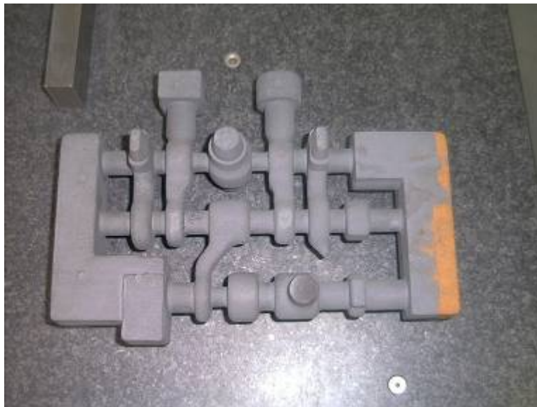
Figure 1. Hydraulic valve body core is shown in the above figure.
