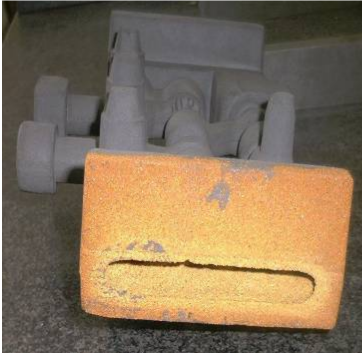
Figure 2. This illustrates the Shell core invest method.
