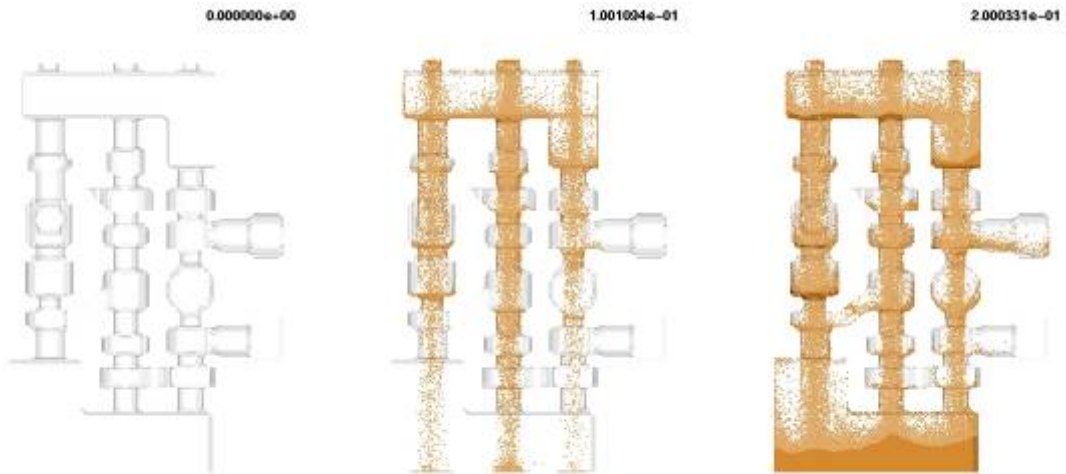
Figure 11. This illustrates core filling sequence.
